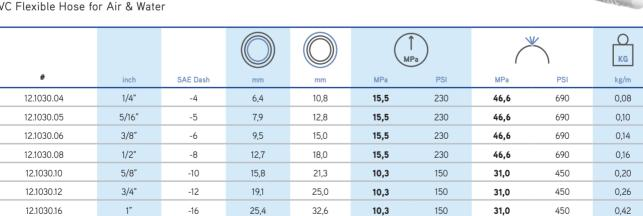
INNER TUBE: transparent PVC, highly flexible, resistant to abrasion INTERNAL SURFACE: smooth, passage facilitator
